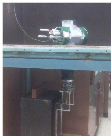
Figure 2: The glove box with the moveable mechanisms and bellows system below. The calorimeter holding vessel and calorimeter is pictured attached to the metal rod that extends through the floor of the cast iron glove box and connects to the bellows system.
