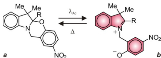
Figure 1. Opening of an oxazine ring (a) to form a zwitterionic isomer (b) under illumination at an activating wavelength.
