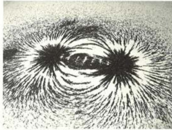
Fig. 5.6. Magnetic lines of force shown by iron filings sprinkled on paper over a magnet. (Courtesy of Windell H. Oksay / www.evil-madscientist.com.)
